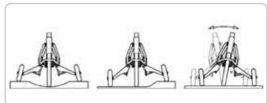
The adjustable suspension intensity and the dynamic stabilizers ensure traction in any riding situation and balanced travel on bends
