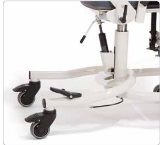
Seat tilt is executed with the aid of a gas pressure spring and the height adjustment by foot pedal
